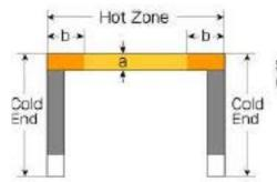
Standard length of the low temperature area (b) shall be 1.5 times of the heating element diameter (a).
